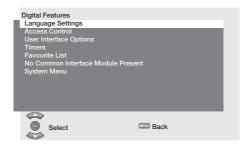
You can select the menu headings with **Up/ Down** movement buttons to make settings.
